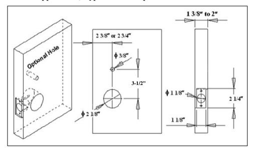
Note: While most of these dimensions are typical for all locks, the distance between the small hole for the optional upper support post and the center of the large lock hole varies with model. Model E6 is shown here.
